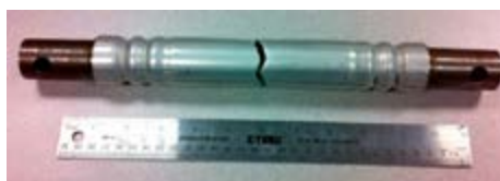
Figure 1. Steel nodes crimped on an aluminum tube and tested in tension.
