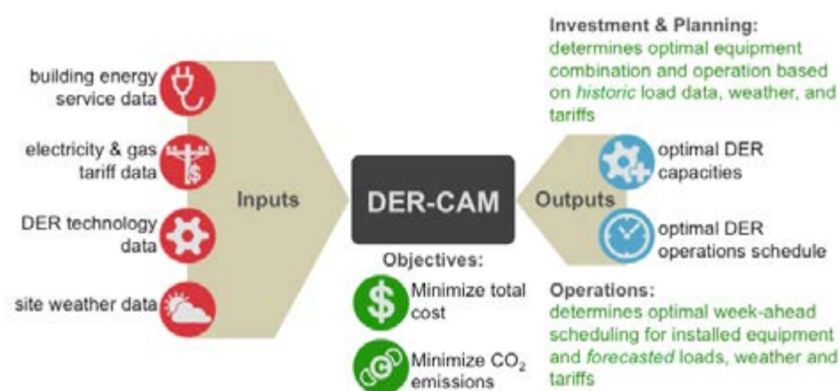
Figure 1. Basic DER-CAM data flow, with key inputs to the left, outputs to the right, and objectives in the center.
