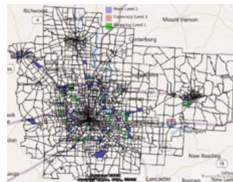
Figure 1. PEV charging infrastructure location optimization model results for central Ohio.
