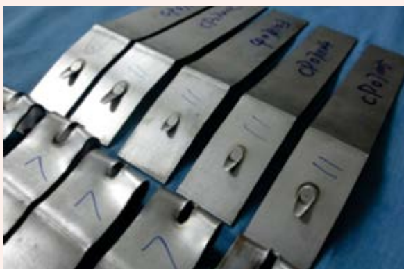
Post-test specimens help characterize the failure mechanisms of crash analyses of high-strength steels.
