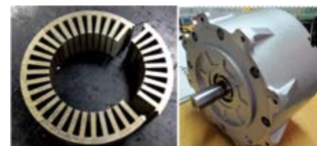
Figure 2. Left: Prototype amorphous iron stator core. Right: Completed machine.
