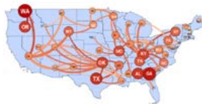
Figure 2. Optimized state-level water consumption and water flows embodied in interstate trade of alternative fuels. Size and color of circles indicate the amount of water consumption related to producing designated fuels, including fuels consumed within the states and those transported to other states. Lines go clockwise from states producing to states consuming designated fuels. Line color indicates the amount of water embodied in interstate trade of fuels.
