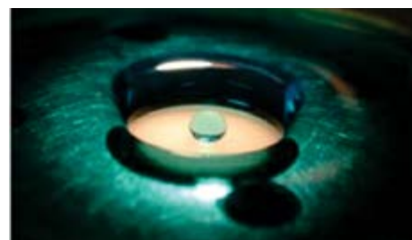
Figure 2. Water drop sitting on top of a circular superhydrophobic surface surrounded by water.
