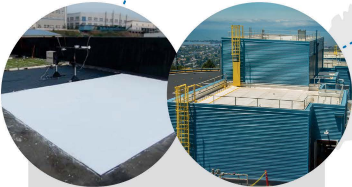
Black, white, and garden roofs being tested at a building in Chongqing, China (left), and cool roof technologies being tested at FLEXLAB at Lawrence Berkeley National Laboratory (right)
