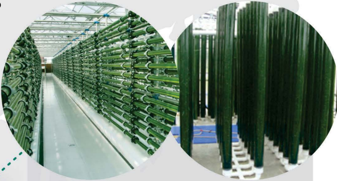
Microalgae testing at the ENN research facility in Langfang, China (left), and at Duke Energy's East Bend Station, Kentucky (right), demonstrating the use of microalgae for CO 2 capture at coal-fired power plants and developing cost estimates for the technology
