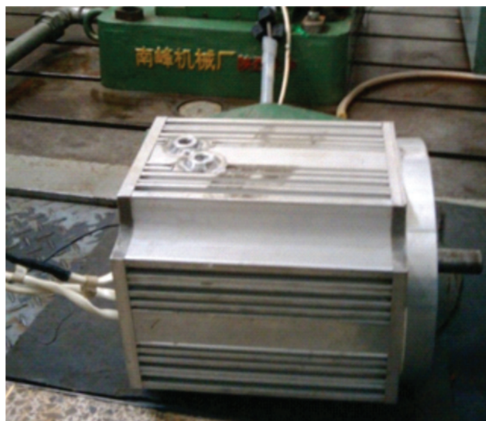
A sample motor of amorphous metal material, 20 kW
