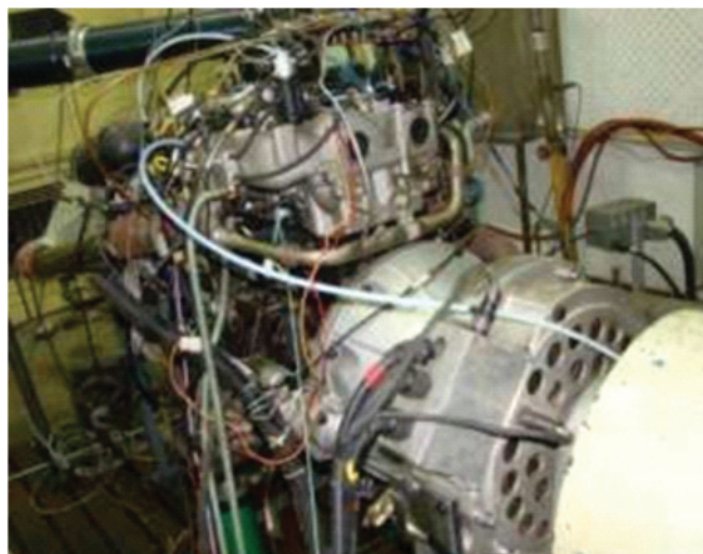
Emission and fuel economy performance test bed with PCCI-CI and CI + ISG motor
