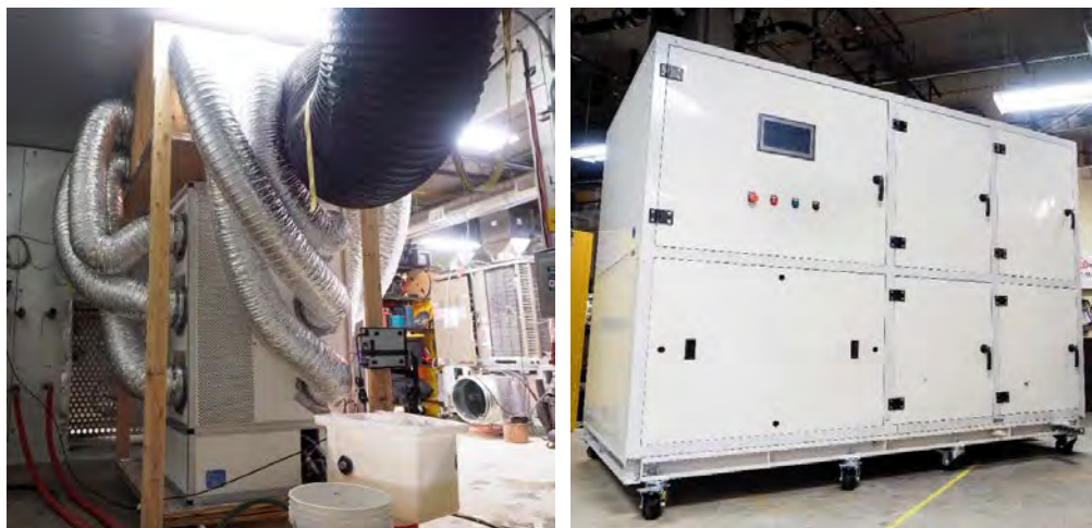
Figure 2: Nexajoule SWEC installed in the environmental chamber (left), Tsinghua SWEC in the WCEC laboratory (right).
